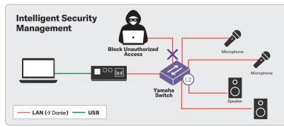
The SWX2310P-28GT includes built-in RADIUS server functionality to augment VLAN capabilities. By setting up one switch as a RADIUS server and linking other switches to it, unauthorized network access can be effectively blocked, ensuring enhanced security even in complex large-scale installations. Device authentication can be quickly and easily configured via a web-based GUI.
