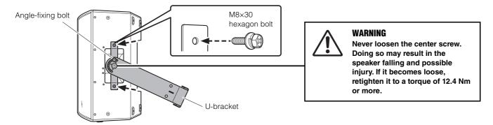
3. Use a wrench to temporarily tighten the angle-fixing bolts on both sides, and install to the wall or ceiling.
