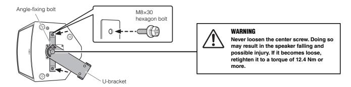
3. Use a wrench to temporarily tighten the angle-fixing bolts on both sides, and install to the wall or ceiling.
