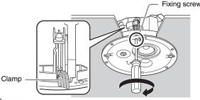
· Do not over-tighten the attachment screw. Otherwise, the attachment screw and clamp will break.
