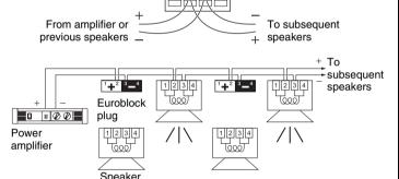
For this method, cables are connected to terminals 2 and 3 of each
