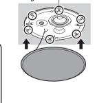
The grille may fall down if it is attached inadequately. Attach it firmly. Incorrectly attached Correctly attached
