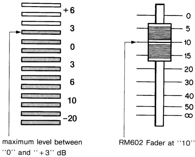
The REC LEVEL control on the deck can be used to optimize the fader setting, as can the level control on the instrument used—in this case the RX15.
