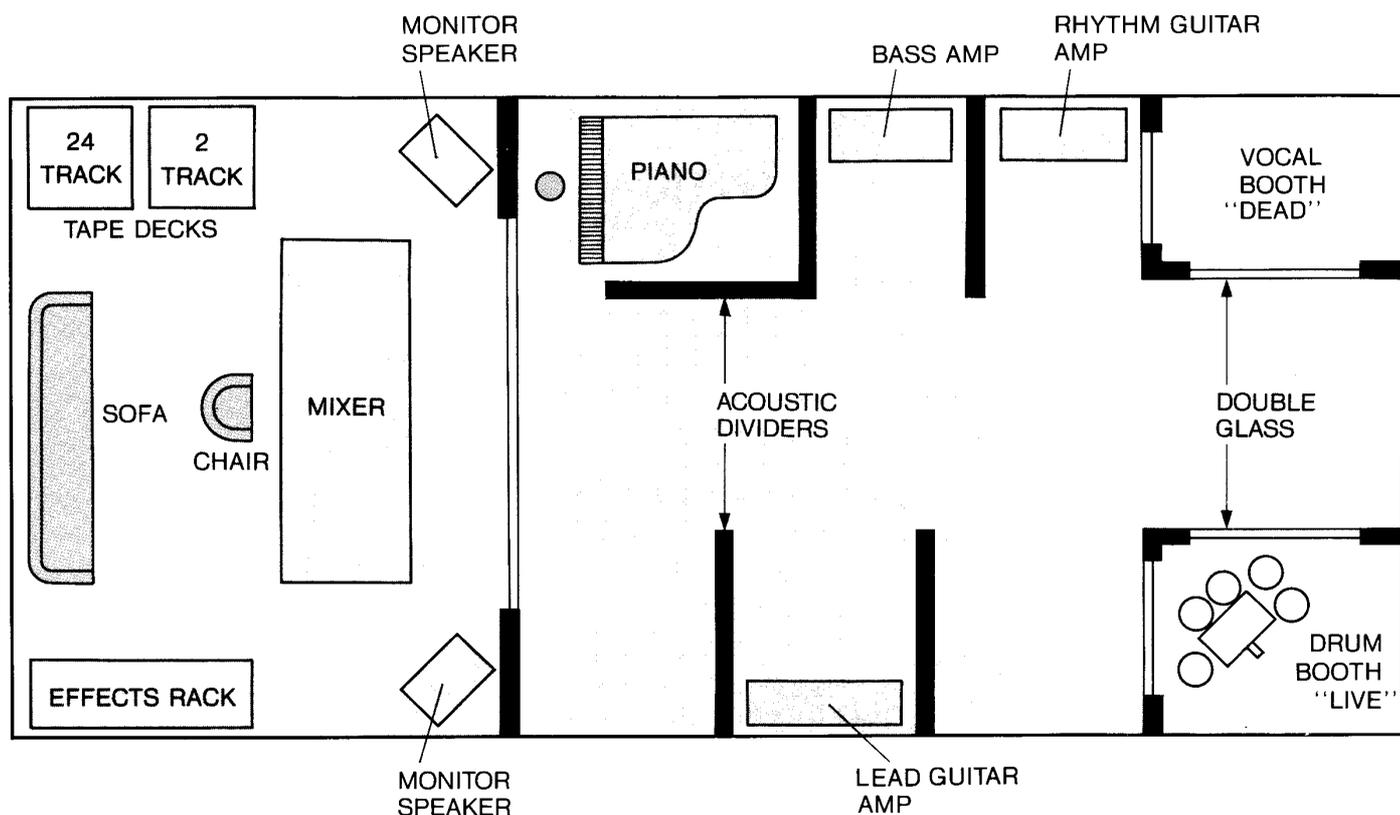
Floor plan of professional multitrack recording studio
