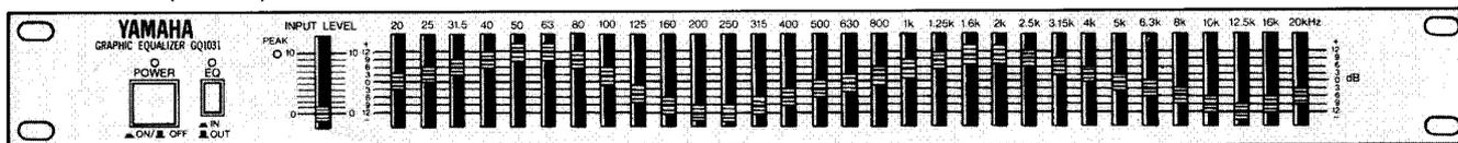
The 31 faders immediately show you what kind of EQ you are applying—a graphic representation of an audible phenomenon. “Equalizer” comes from the original function of these devices—to make the recorded sound “equal” in tone to the original sound, though nowadays the aim is often to make it better than the real thing!
