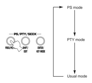
The name of the station being received is displayed. If the station is not an RDS station, "NO PS" flashes on the display and then returns to usual mode.
