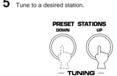
To tune to a higher frequency, press the **UP** button once. To tune to a lower frequency, press the **DOWN** button once.
