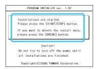
Press the [START/STOP] button to start installation.
