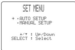
If ^ is pressed when AUTO SETUP is selected, or if v is pressed when MANUAL SETUP is selected, SET MENU will be closed. Press ^ / v to open SET MENU again.
