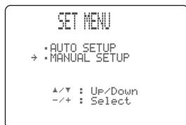
If  $\wedge$  is pressed when AUTO SETUP is selected, or if  $\vee$  is pressed when MANUAL SETUP is selected, SET MENU will be closed. Press  $\wedge$ / $\vee$  to open SET MENU again.
