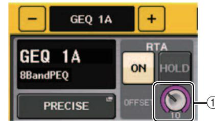
① **Offset gain (RTA METER window, HPF/EQ window, GEQ window, 8BandPEQ window)**
