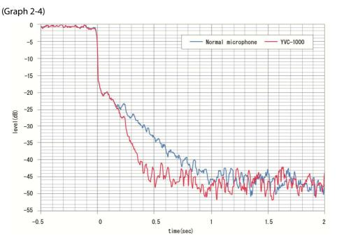
As shown in Graph 2-4, a measuring sound (white noise) was reproduced from a supposed person's location and then the reverberation convergence time from the reproduction stop time (0 sec in the graph) was compared between a normal microphone (without dereverberation) and YVC-1000's microphone. It is clear from the results that YVC-1000's reverberation converges more quickly than the normal microphone's.
