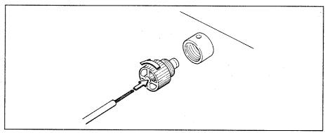
Splay the strands as shown, then screw the wire holders back on.
