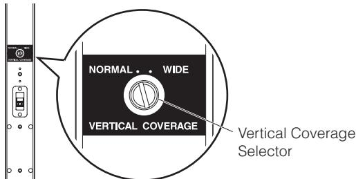
At this time, when you want to expand the area of coverage downwards, set the switch to WIDE.
