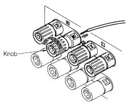
The speaker connection wires should be no longer than necessary.
