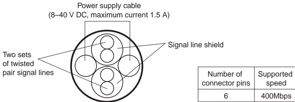
Since the six-pin cables are able to transmit power, power can be distributed between nodes of the network. Nodes can be classified by how they handle power.
