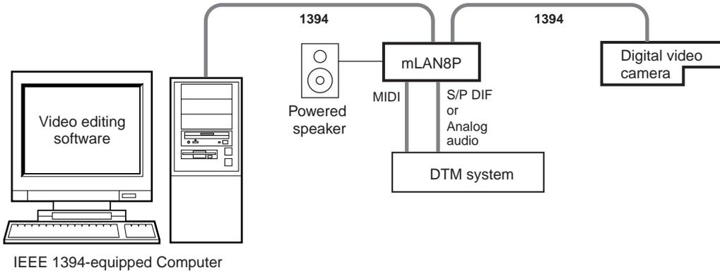
**NOTE** The signals from the digital video camera are not recognized by mLAN8P but passed through it to the computer.
