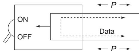
When the power is turned off, the nodes can still obtain power and function as bus relay. When the power is turned off, the nodes can still obtain power and function as bus relay.
