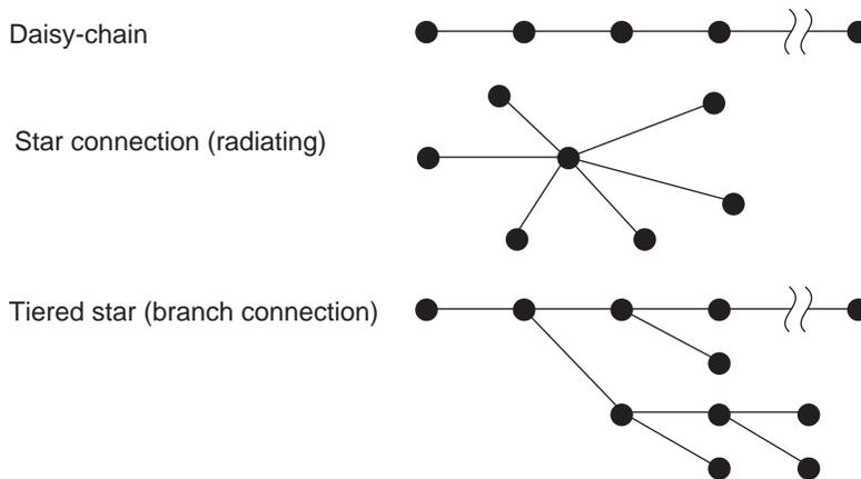
In these topologies, it is possible for any node to be seen from any other node as being in a “tree” structure. In this case, the single selected node is called the “root node.” As the name suggests, the tree structure is similar to the branched form of a tree, but is normally drawn upside down from an actual tree. Thus, the “root” will be depicted at the top of the diagram. As shown in the following diagrams, any node in the topology can be the root node.
