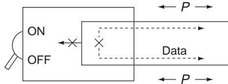
When the power is turned off, the nodes do not obtain power and cease functioning as bus relays.
